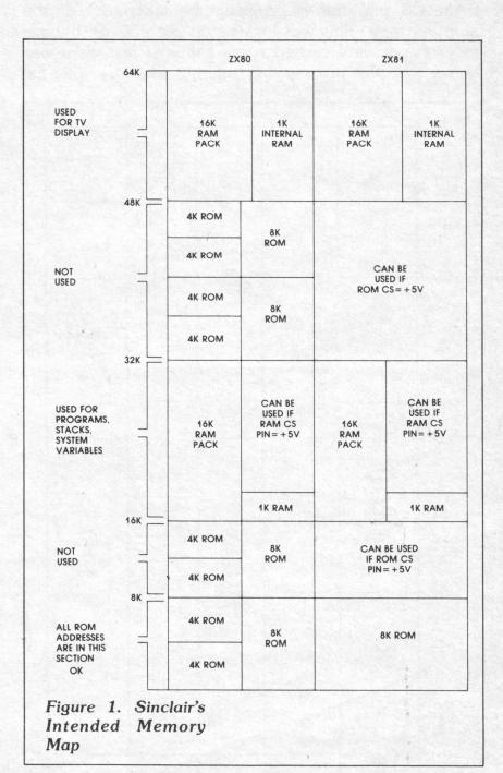
pin called RAM CS on the expansion board, the RAM could be turned off. Sinclair included this feature in their design because some method was needed to turn off the 1K of internal RAM when the 16K RAM pack was fitted on the back.
