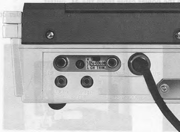
Rear panel of the MZ-700 series computer
