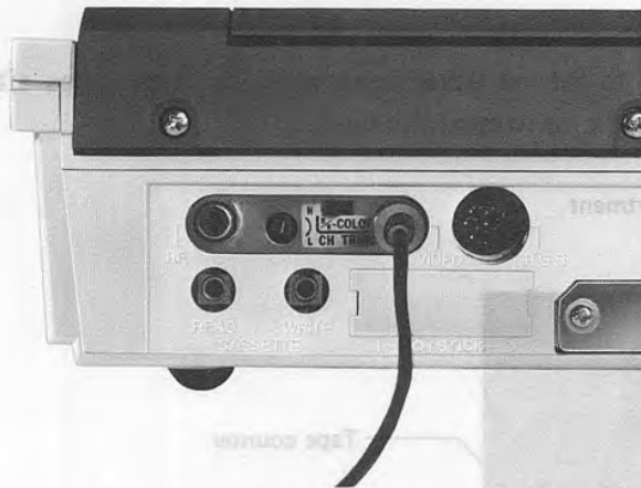
Rear panel of the MZ-700 series computer
