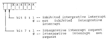
When the inner interpreter examines INTFLAG and handles interrupt signal, it fetches CFA (code field address) in INTVECT and begins to execute the interrupt handling program.
