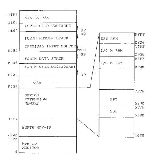
FORTH-MPF-IP uses a memory space of 8k bytes, from \$2000 to \$3FFF. The system will insert the word TASK at F000 after the machine is turned or or the execution of the cold start (using the word COLD). The user's dictionary grows upward from F00B. For more details about TASK, please see Chapter 9. \$FE00 through \$FEB0 is allocated for user variables, consult appendix D.
