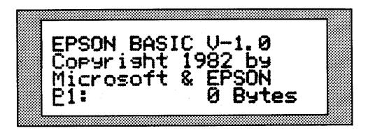
When BASIC is executed, the programme area No. 1 is always selected. The message "0 Bytes" following "P1:" indicates the length of the programme stored in the current programme area. In this case, as no programme has been stored in program area No. 1, the value displayed is "0" bytes.
