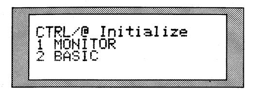
The menu displays numbers and the functions (i.e., programme names) which can be executed when you press the corresponding numeric keys. When power is applied to the HX-20 for the first time, only two functions will appear on the LCD screen as shown above. "CTRL/@" at the uppermost line of the display indicates that you must press the while holding down the CTRL key.
