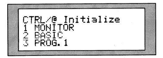
5 programmes registered in the menu are numbered 3 through 7, respectively. Any of these programmes will be executed directly (without using LOGIN and RUN commands) whenever you press the numeric key corresponding to the programme number.
