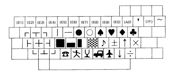
NOTE: E0 through E9, A0 and 7F shown in parentheses in the above figure are character codes in hexadecimal numbers and can be input by pressing the corresponding keys while holding down the GRPH key. The character codes for ¶ and ~ are 60 and 7E, respectively. (See Chapter 8, "Definition of Graphic Pattern" in the HX-20 Operation Manual.)
